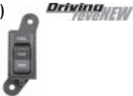
Fuel Tank Selector Switch
