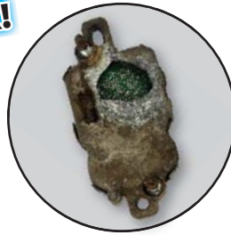
Original Aluminum Housing – Extremely failure prone due to corrosion
